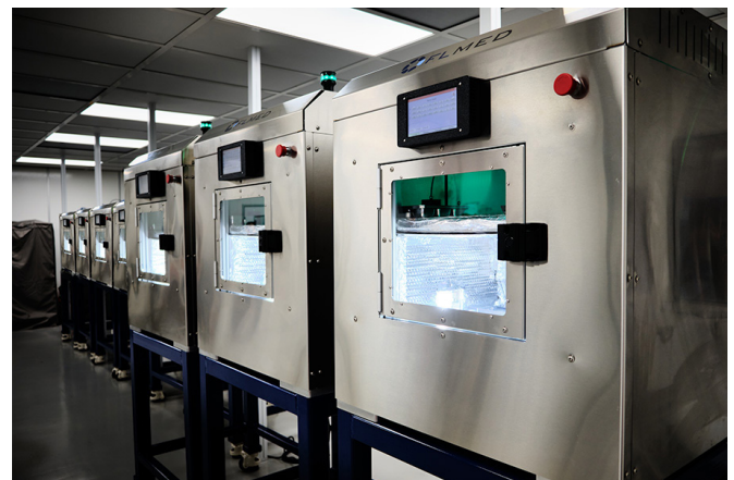
Inspire is manufactured on Curiteva’s proprietary 3D printers, reportedly the first FFF printer to consistently print PEEK implant structures.
