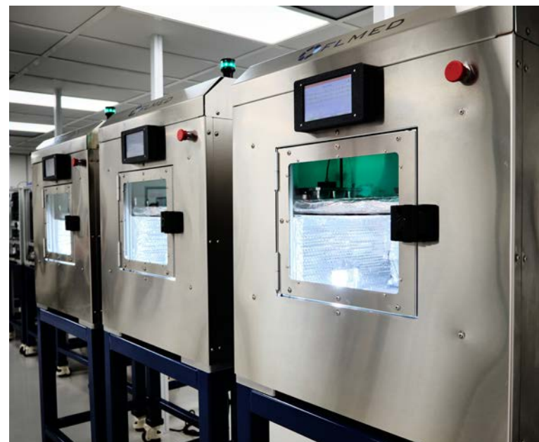
Curiteva currently produces implants with ten printers. Depending on the size, production takes between 15 minutes and several hours.
